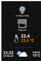
Smart Touch Panel can communicate with other wireless inohom products as well as realize automation management with 4 internal relays and 0-10V analog output.
